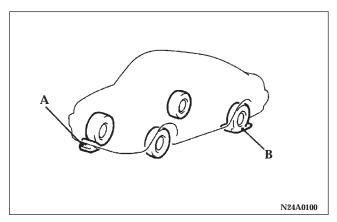
4. Apply a chock or block (A) at the tire diagonally opposite the tire (B) to be changed.
